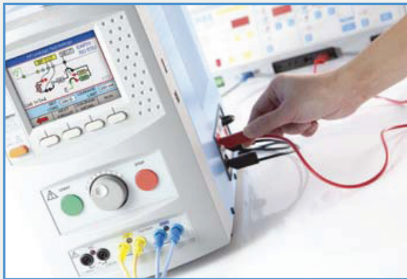
Figure 13: Connection panel on the Rigel Uni-Therm
