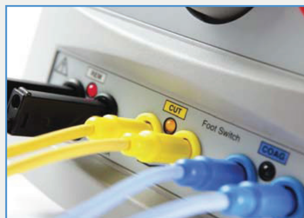
Figure 16: Connection panel for the cut and coag footswitch control on the Rigel Uni-Therm
