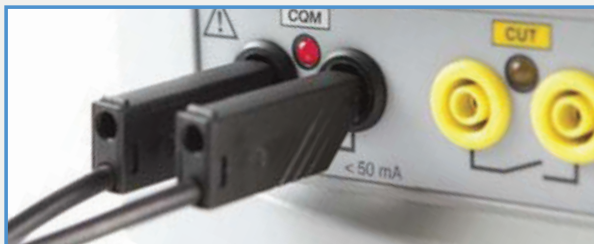
Figure 9: Connecting Rigel Uni-Therm to the CQM circuit
