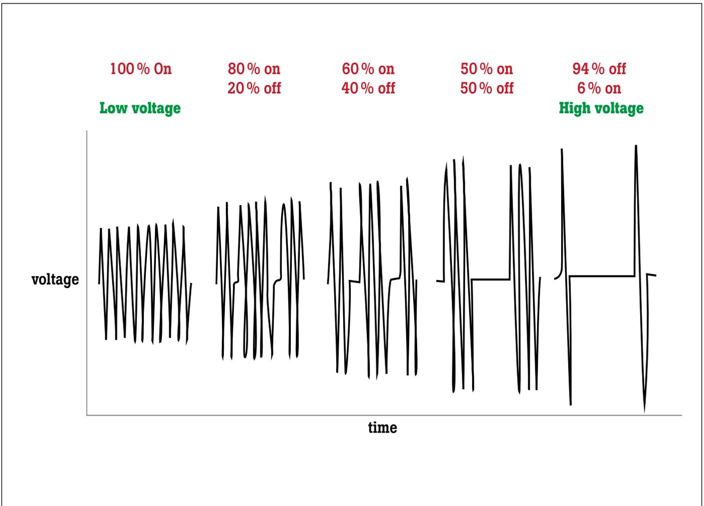
**Figure 3:** Electrosurgical waveforms
